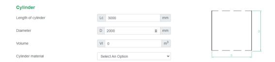
Note that Amphora automatically determines the number of sections to divide the cylinder. This is based on the 'length of cylinder'.
