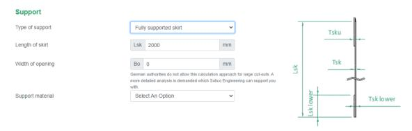
When you select a fully supported skirt, an opening can be introduced. When an opening is present, enter the 'width of the opening', otherwise enter 0 to remove this option.
