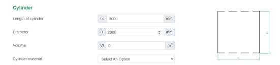
Note that Amphora automatically determines the number of sections to divide the cylinder. This is based on the 'length of cylinder'.
