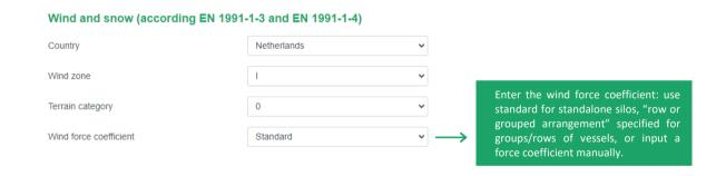
If your vessel is located outside the available countries in Amphora, you can select the option "user input" from the "country" pull-down menu. This allows you to fill in the values of the extreme wind pressure and snow load on the ground for the location. These pressures can be calculated according to the national annex of the EN1991-1-3 and EN1991-1-4 of the specific country.
