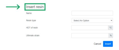
Please note that Amphora does not verify if the resin used aligns with EN13121-2. The user must ensure compliance between the resin of the liner and structural laminate. If information in EN13121-2 is insufficient, seek resin advice from your resin provider.
