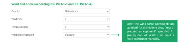
If your vessel is located outside the available countries in Amphora, you can select the option "user input" from the "country" pull-down menu. This allows you to fill in the values of the extreme wind pressure and snow load on the ground for the location. These pressures can be calculated according to the national annex of the EN1991-1-3 and EN1991-1-4 of the specific country.
